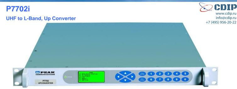
The 19-inch, 1RU rack mounted P7702i block up converter unit from Peak Communications is designed to typically take the incoming UHF signal and produce an output at L-Band that is suitable for further conversion by a P7001 converter or for direct connection to a receiver in a down link chain.
